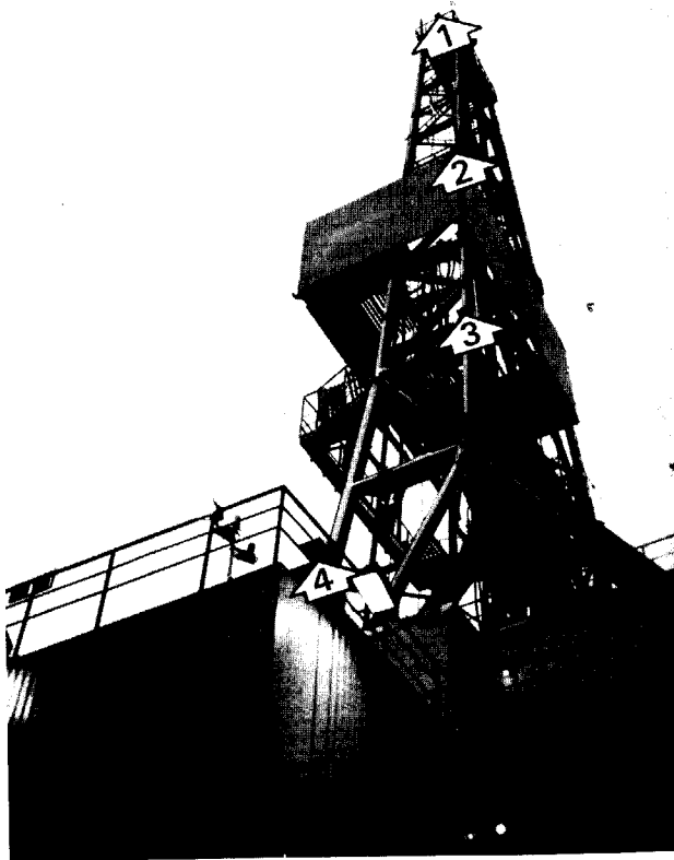
Figure 3. Locations of Rosemount ice detectors on derrick. Heights (above deck) are 1 - 180 ft; 2 - 120 ft; and 3 80 ft. Number 4 is on the railing above the diving bell area, about 20 ft above deck.
