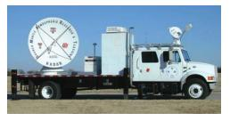
One of the mobile 5-cm SMART-Rs was recently modified to perform simultaneous transmit/receive dual-polarization measurements. As a research radar, the SMART-R can transmit real-time data products back to the Hazardous Weather Testbed in Norman, OK, where researchers and forecasters are testing new techniques.
