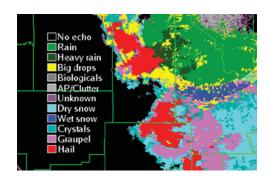
Dual-polarization technology ,when added to the WSR-88D radar network, will help forecasters identify different types of precipitation within radar data.
