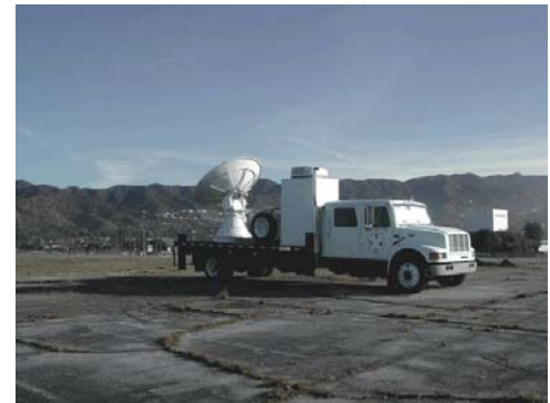
The SMART-R being used near the Day Fire burn area in California to study debris flows. (photo: NOAA)
