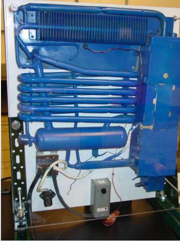
Absorption Heat Pump Cycle
