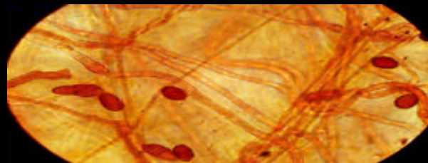
Fungal growth from evaporator A - swab sample
