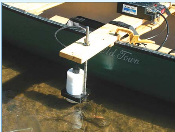
Acoustic Doppler current profiler mounted on canoe for shallow-water flow measurements. [Photo by Gary T. Fisher, U.S. Geological Survey]
