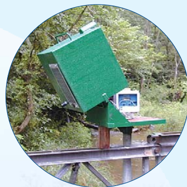
Data collection and transmission using Sutron data recorder and AirLink data-transmission equipment. [Photo by Richard W. Saffer, U.S. Geological Survey]
