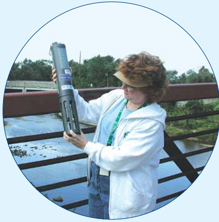
USGS scientist inspecting a probe used for continual measurement of pH, dissolved oxygen, turbidity, and specific conductance. [Photo by Robert J. Shedlock, U.S. Geological Survey]
