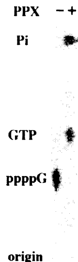
FIG. 4. Degradation of ppppG by PPX. \alpha -[ 32 P]ppppG (20 pmol) was digested by yeast PPX (500 units) at 37°C for 60 min. The TLC plate was developed with 1.5 M KH 2 PO 4 (pH 3.5) and autoradiographed.
