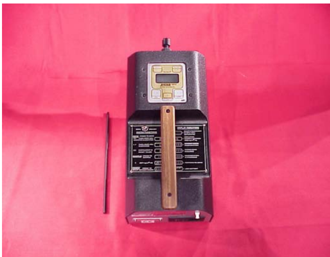
Figure 13 A-12. Jerome Model 431X Mercury Vapor Analyzer
