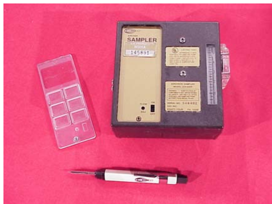
Figure 4-1. SKC Model 224-44XR Sampling Pump
