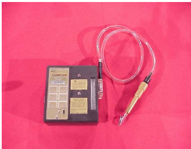
Figure 9-1. Sorbent Tube Sampling Train (SKC Pump)
