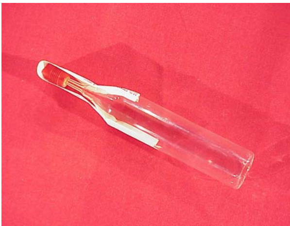
Figure 12-4. 50 mL Vacuum Bottle with Sample Seal
