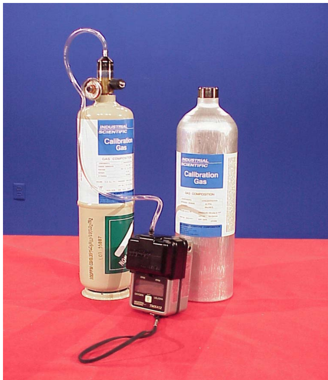
Figure 13A-2. Calibration of TMX-410 and TMX-412 Instruments
