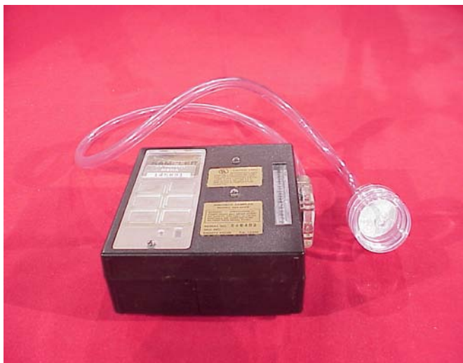
Figure 7-2. Welding Fume Sampling Train
