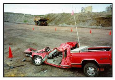
smaller vehicles is also an effective warning device and, when coupled with a properly extended flagpole and flag, provides excellent warning to equipment operators.
