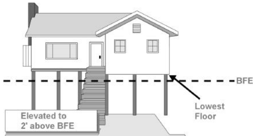
Figure 7-12. Repaired—elevated 2 feet above BFE; actuarial rate: $216
