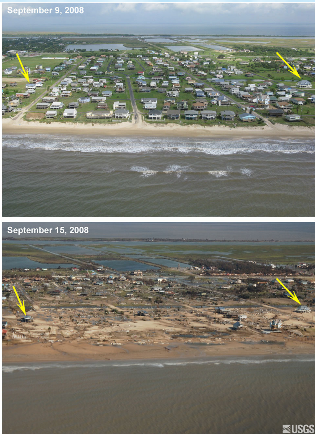
Figure 3. Aerial photography of the Bolivar Peninsula on September 9, 2008 (top) and September 15, 2008, two days after landfall of Hurricane Ike (bottom), showing storm surge damage.
