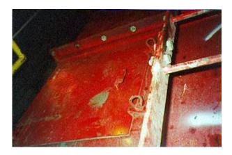
Some simple modifications to these access doors would prevent this type of accident. Installing a piece of metal grating or mesh across the door opening would allow visibility and access into the chute, while preventing any significant flow of material out of the access door.
