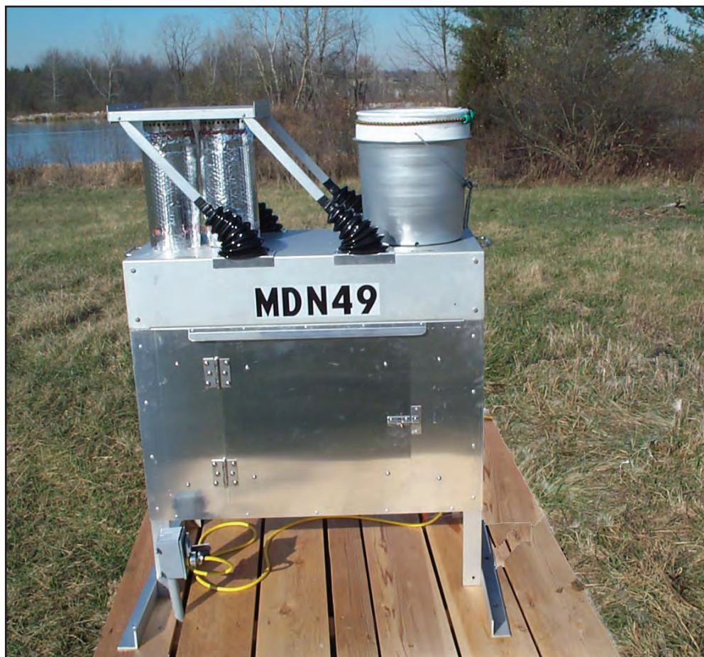
Figure 11. Automated precipitation sampler for mercury in precipitation at monitoring station IN20 at Roush Lake near Huntington, Indiana.
