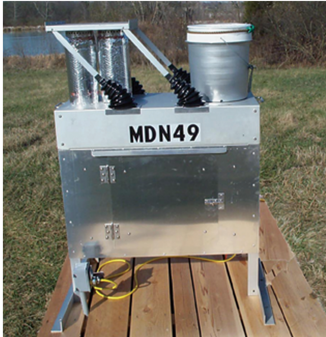
Figure 8. Automated precipitation sampler at monitoring station for mercury in precipitation in Indiana.
