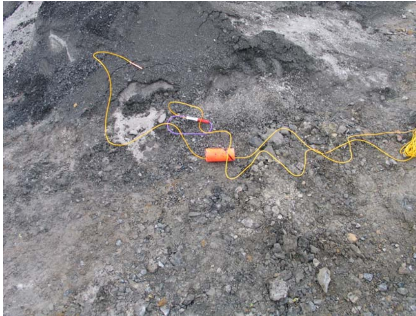
Figure 5 - Orica UNI Tronic™ 335 electronic detonator and booster
