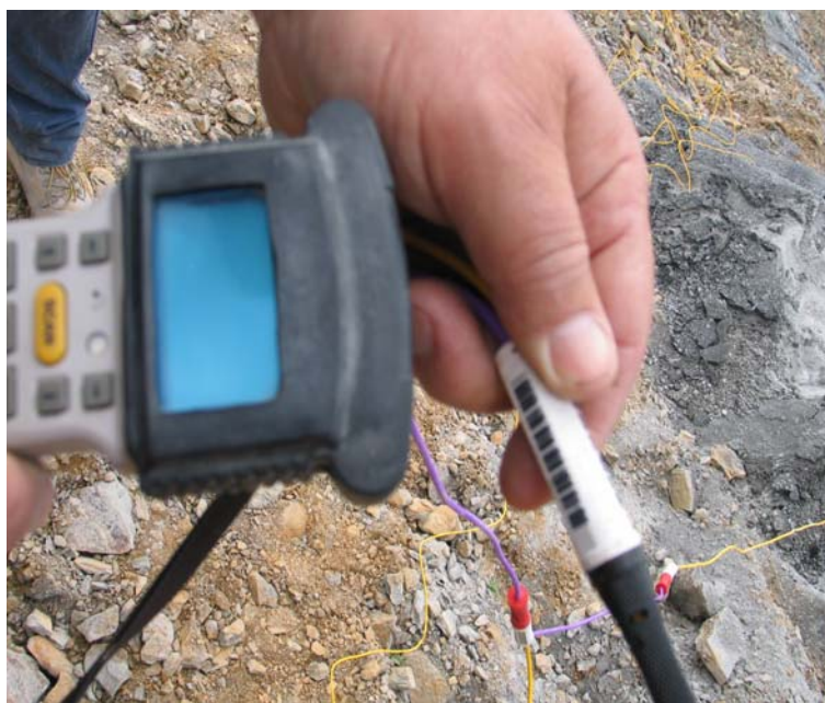
Figure 3 – Orica UNI Tronic™ 335 Electronic Detonator Assembly
