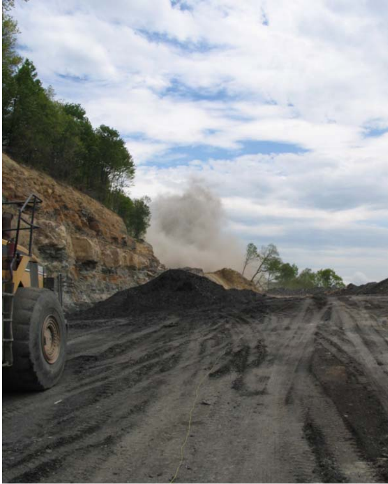
Figure 15 – Firing of the blast at the mine site using the Orica UNI Tronic™ Blast Box
