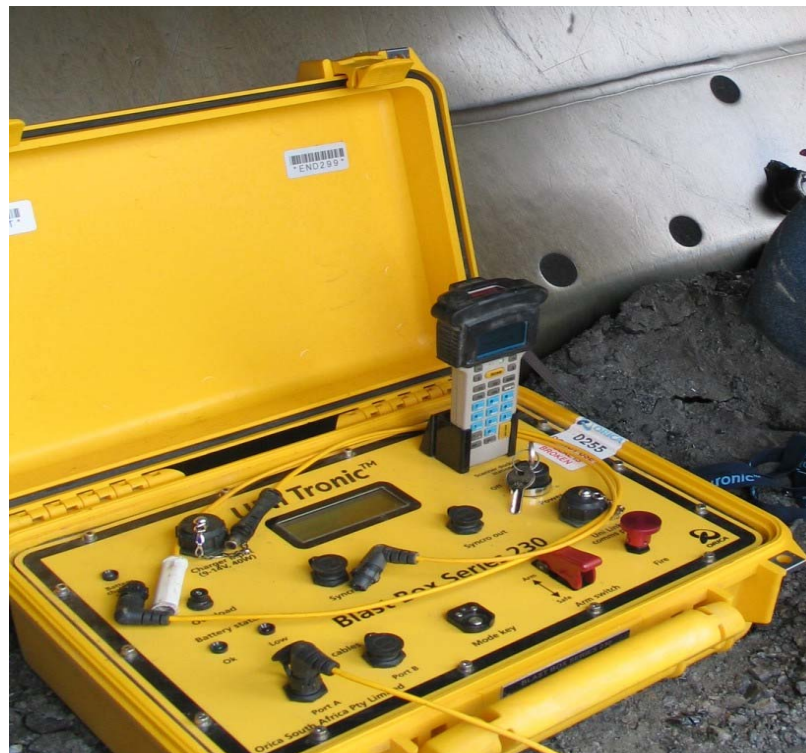
Figure 8 -- Orca UNI Tronic™ Blast Box with the Scanner inserted to download electronic detonator information
