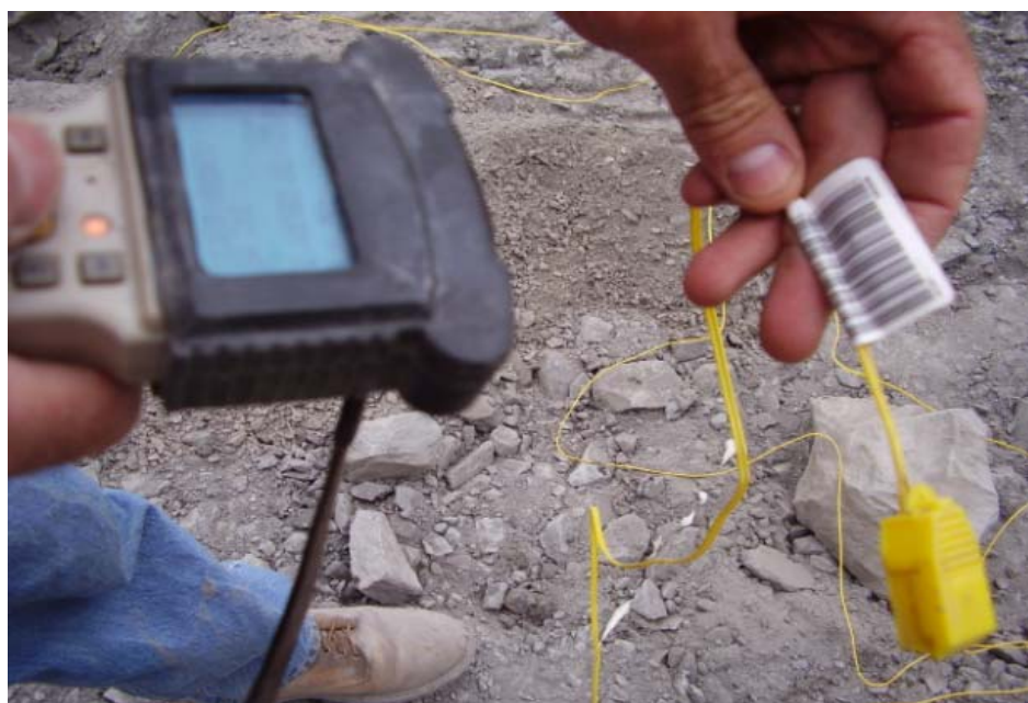
Figure 10 – Orca UNI Tronic™ Scanner used to read an electronic detonator (Unitronic™ 500) bar code ID
