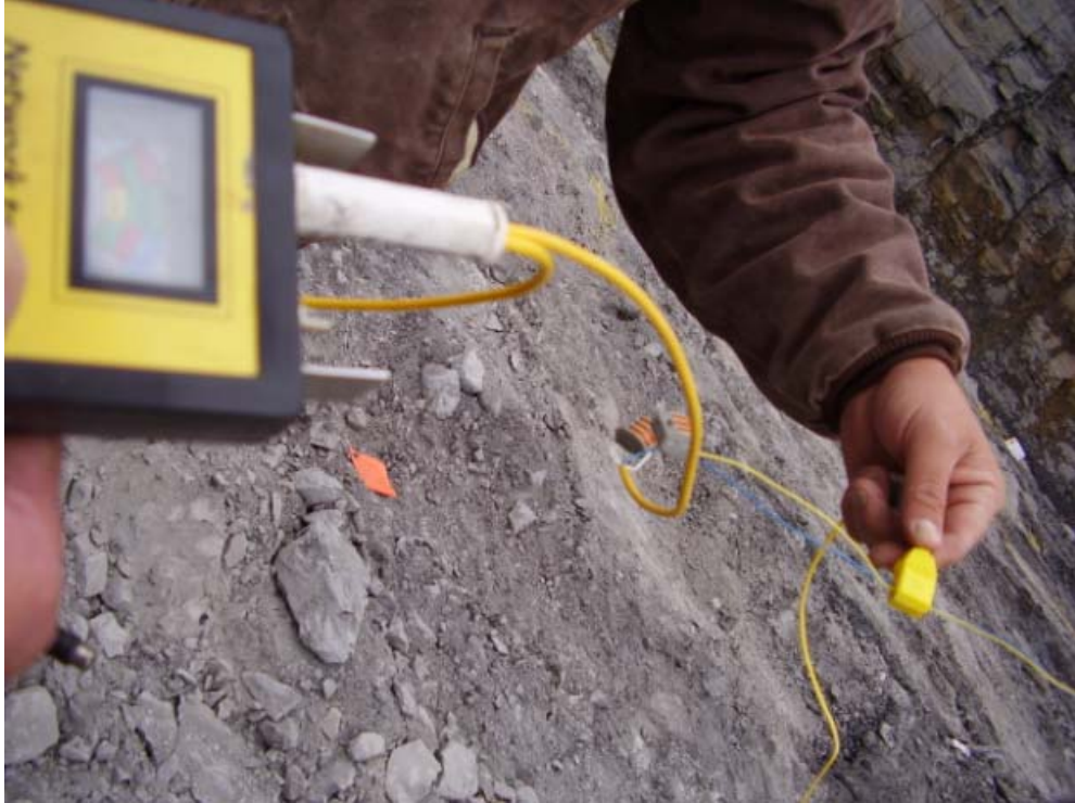
Figure 12 - UNI Tronic™ Network Tester used to test a UNI Tronic™ 500 electronic detonator
