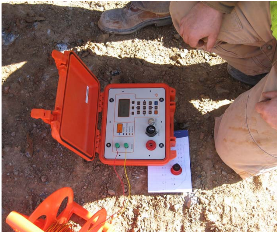
Figure 9 - Connection into the Digishot™ Blaster for checking the blast layout and programming of the blast
