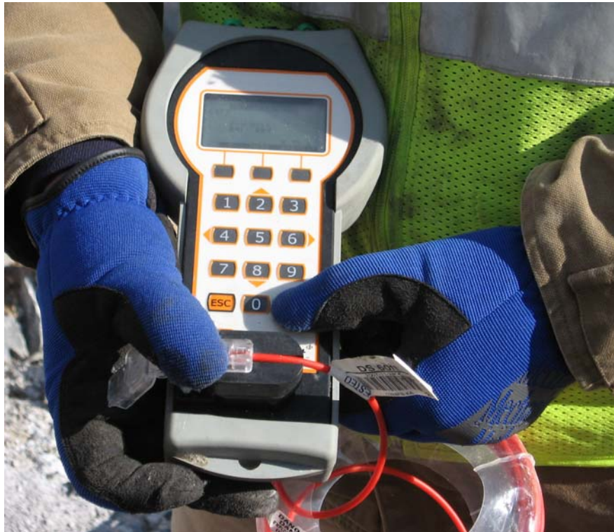
Figure 8 - Inserting the electronic detonator wire into the Digishot™ Tagger
