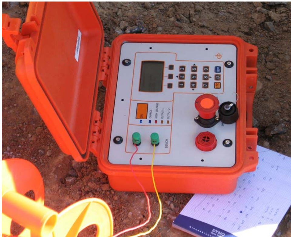
Figure 10 - The Digishot™ Smart key for initiation of the blast inserted into the Blaster
