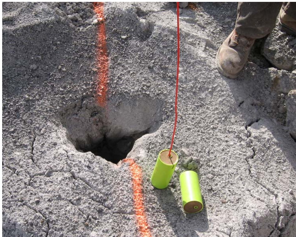
Figure 7 – Placement of Digishot™ electronic detonator into a booster
