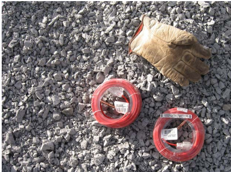
Figure 6 – Electronic detonators & down-hole wire coil for connection & tagging
