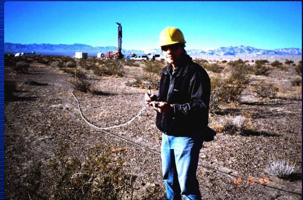
UZB-3 borehole (115-m deep, 15-cm diam.) – ~2 km of cables & tubing ... “The White Mamba”
