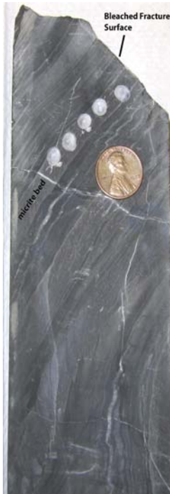
Figure 48. Photo of how individual limestone beds were sampled for isotopic analysis progressively away from a bleached fracture surface. Samples 00NZ158_2032.5 MT1-5. Coin: 19 mm. See Text for discussion.
