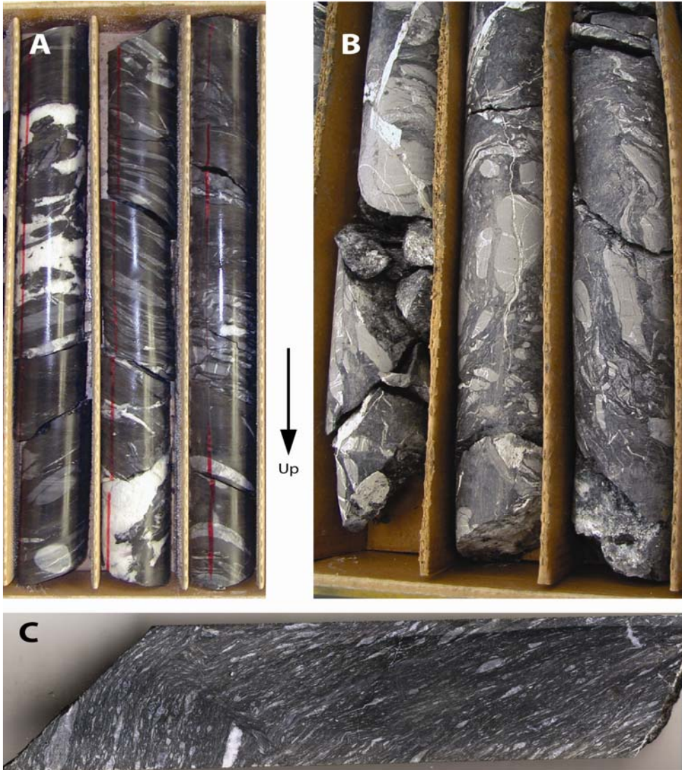
Figure 8. Examples of the sedimentary breccia unit from Turquoise Ridge. A. Gray micrite beds from the lower part of the sedimentary breccia unit that have been stretched into disc-shaped boudins. The boudins are interpreted to be parallel to primary bedding and to have formed by stretching of more competent limestone layers during compaction and slumping of the carbonaceous mudstone and limestone unit before it was completely lithified. Drill core from hole 00NZ158 at depths of 2804.5 to 2810 feet. B. Breccia from the lower part of the sedimentary breccia unit consisting of subangular to subrounded fragments of gray micrite supported by non-calcareous carbonaceous mudstone. Drill core from hole 99NZ023 at depths of 2618 to 2624 feet. C. Example of fine-grained, shear-textured breccia that originated from a thin-bedded interlayered sequence of carbonaceous mudstone and limestone. Original bedding is marked by stretched boudins of gray micrite, supported by non-calcareous, carbonaceous mudstone. Hole TU00929 448.8 feet, in the upper part of the sedimentary breccia unit.
