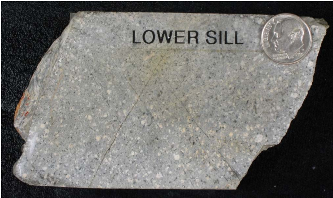
Figure 13. Drill core showing main dacite porphyry dike of Cretaceous age at the north end of Turquoise Ridge. Coin: 17.5 mm.
