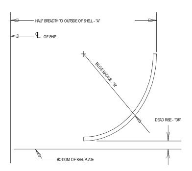
NOTE: During an off center lockage in which the vessel contacts the locks walls, the bilge radius should be free from chamber slopes in the most critical part, as shown in Table of Limiting Drafts of this annex.
