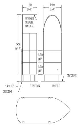
PILOT SHELTER PLATFORMS MAY BE REQUIRED ON VESSELS WITH A MAXIMUM BEAM OF 30.48m (100') OR MORE AND AN OVERALL LENGTH OF 190m (625') OR MORE.
