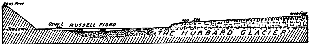
FIG. 20. CROSS-SECTION OF RUSSELL FIOR'D AT HUBBARD GLACIER. VERTICAL AND HORIZONTAL SCALES THE SAME.
