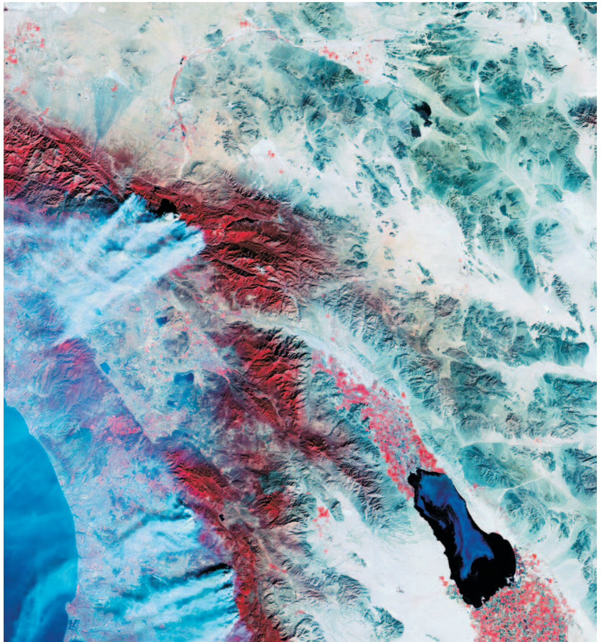
Figure 56. This image of the California fires was supplied by Surrey Satellite Technology from the Disaster Monitoring Constellation. The smoke from the fires is white. The footprint from this satellite is approximately 600 kilometers (km) square, compared to Landsat at 185 km.
