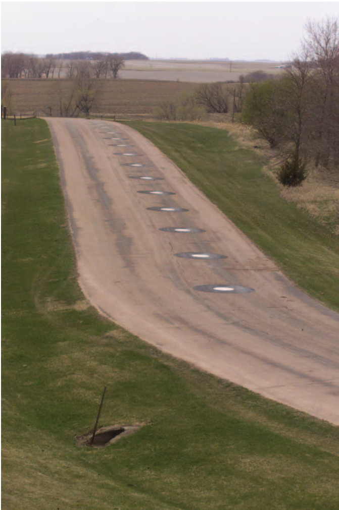
Figure 59. Example of EROS range points for aerial and satellite calibration and validation.
