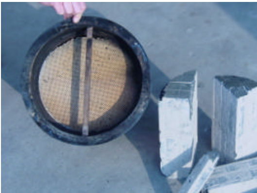
Filter core broken due to vibration at less than 1000 hours, replacement cost at least € 3000.-
