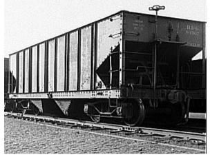
control valve was in the "door open" position and the pressure in the air system had not been released. When a chain holding damaged doors shut was cut with a torch, the doors suddenly opened and pinned the mechanic, who was standing in a service trench under the rail car. The crushing injuries were serious because one door swung open farther than it normally would due to the broken mechanical linkage that was to be replaced.
