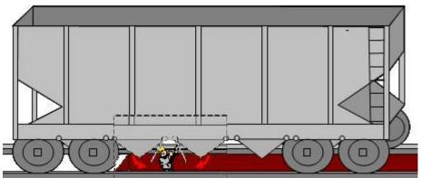
Before working on rail car discharge doors, it is important to dissipate all stored energy that could cause the doors to move. Understand and follow the manufacturer's service/operations manual and be sure to:
