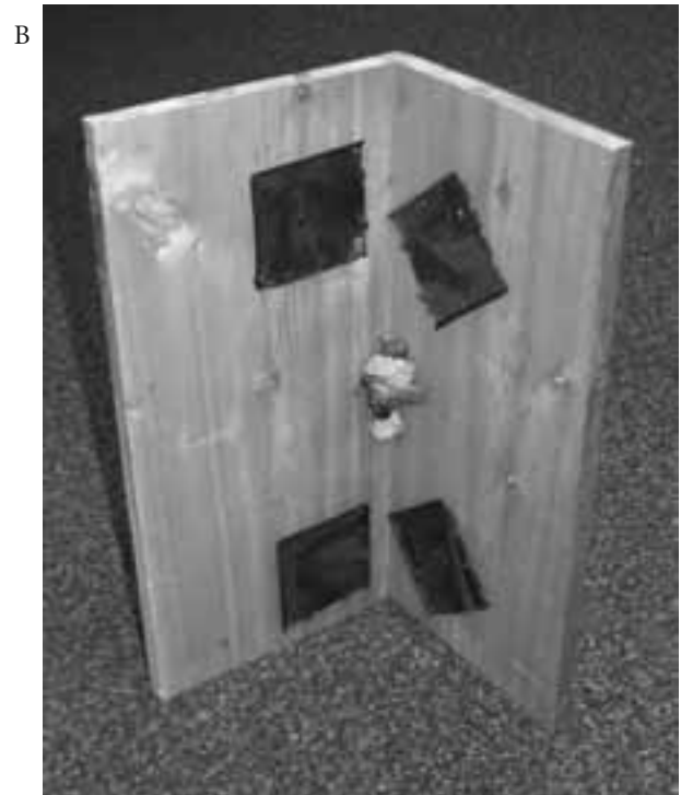
Figure 6.7. Marten cubby that can be accessed from both ends. (A) Cubby is vertically mounted on a tree with a roof installed above the top end (photo by J. Stetz). (B) Glue traps are fitted inside to collect hair on either end of the bait attached at the center of the cubby (photo by K. Kendall).
