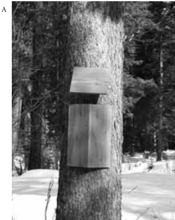
Figure 6.7. Marten cubby that can be accessed from both ends. (A) Cubby is vertically mounted on a tree with a roof installed above the top end (photo by J. Stetz). (B) Glue traps are fitted inside to collect hair on either end of the bait attached at the center of the cubby (photo by K. Kendall).
