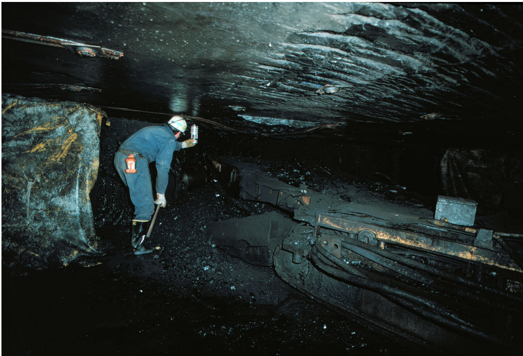
Figure 11. Photograph showing a continuous mining machine in an Upper Freeport coal bed mine, Homer City region, Indiana County, Pa. Continuous miners were introduced in the late 1940's and are currently used to produce over 50 percent of the underground coal tonnage mined in the Appalachian Basin (Reid and Richardson, 1995). (Photograph courtesy of Ronald Stanton, USGS.)
