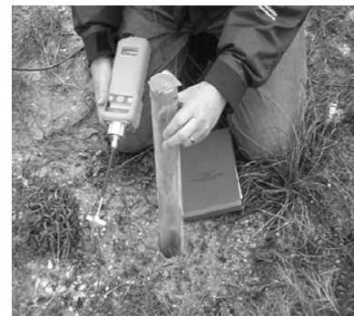
White tip (moisture filter) of hand-held PID (Yellow) is inserted into blue cap of plastic tube that is lowered into augered hole for measurement of VOCs at various depths.
