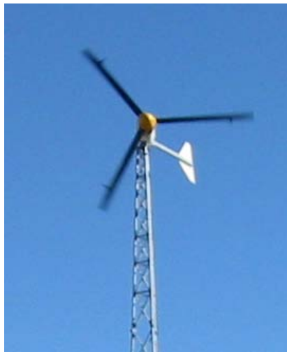
Figure 2-14: 10 kW Bergey Excel-S wind turbine at the NWTC
