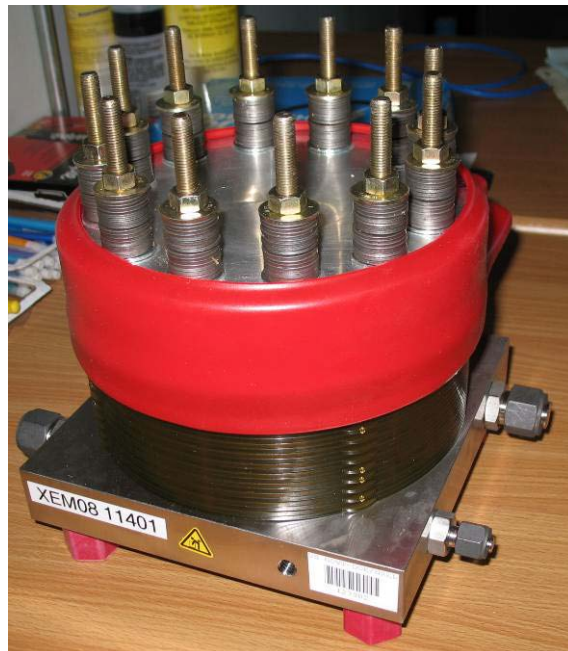
Figure 6-1: Additional 10-cell PEM stack cells to be installed in series with existing 20-cell stack inside E-120 electrolyzer
