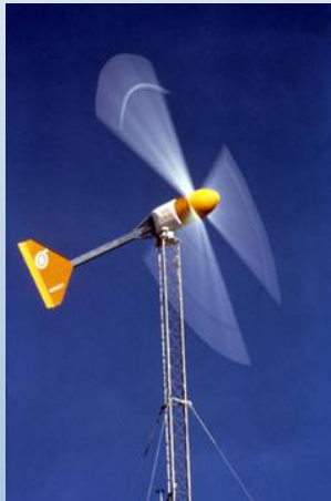
10kW Wind Turbine
