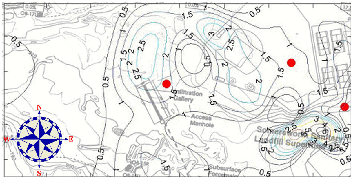
Figure 3-6. The OP-FTIR RPM Methane Concentration Contours Overlaid on the Map of the Somersworth Superfund Landfill.
