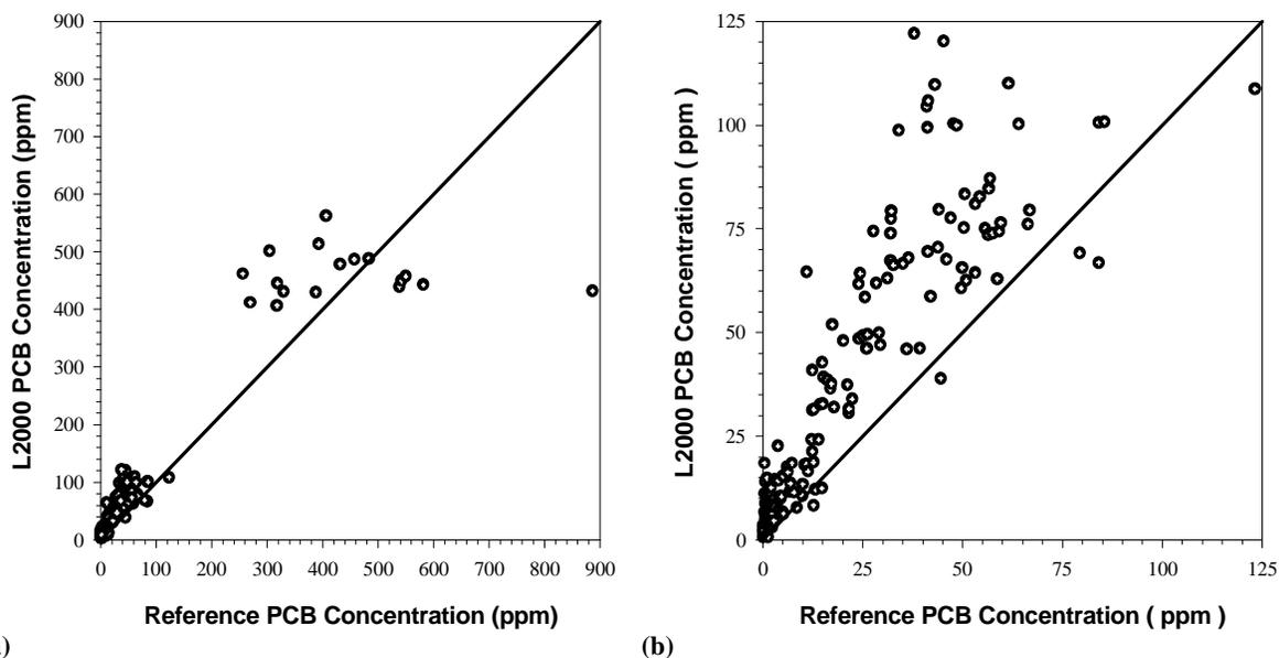
**Figure 5-1. Paired PCB measurements for the L2000 and reference laboratory for (a) all soil samples and (b) soil samples where the reference laboratory results were less than or equal to 125 ppm. Lines denote perfect correlation.**
