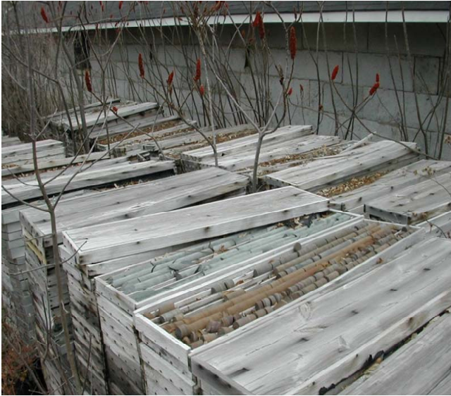
Figure 1 – Drill cores are expensive to obtain, and they – quickly lose their usefulness if not properly sheltered from the elements. (Courtesy of the Maine Geological Survey)
