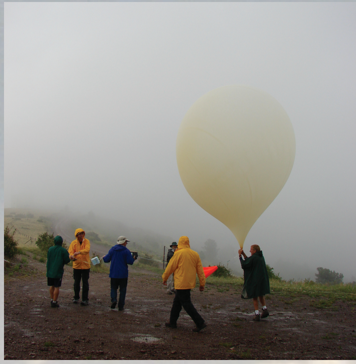
Calm winds on a mountain ridge allow scientists and students to release a balloon and instrument train directly into the storm.
