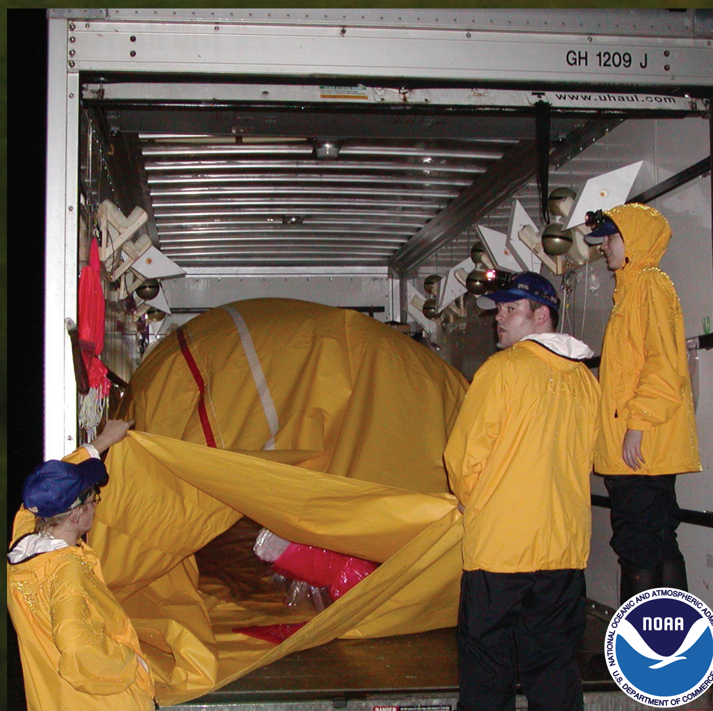
(Right) Crew members in a truck configured as a mobile inflation shelter inflate a balloon and check out instruments for the next flight. Inflating a balloon in its launch tube allows it to survive handling and launch in strong winds.
