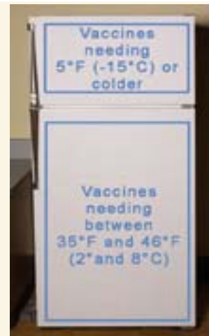
Refrigerator and freezer compartments must have separate external doors.
