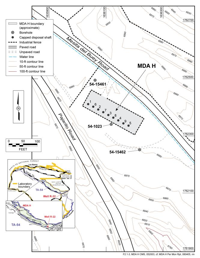
Figure 1.0-2 Locations of vapor-sampling boreholes at MDA H
