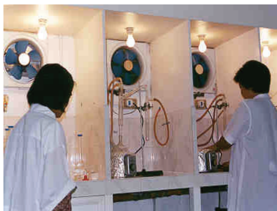
Figure 2. Distillation apparatus used by IMA chemists to digest tissue samples in order to liberate hydrogen cyanide gas, that is then captured as cyanide ion in an absorber tube containing sodium hydroxide.
