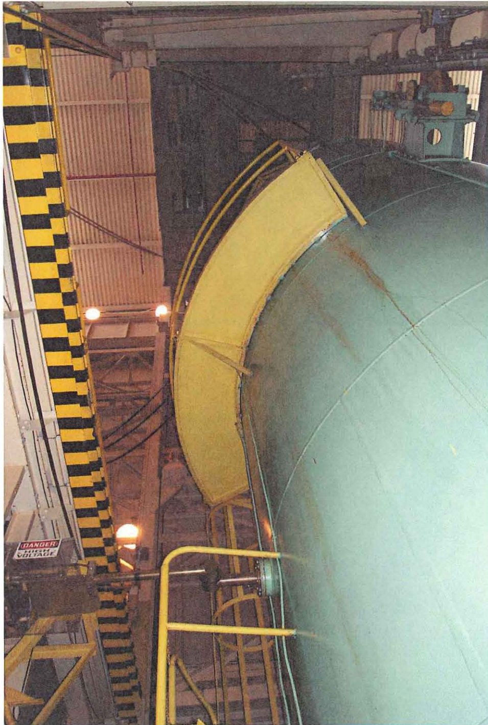
Figure 5. Van de Graaff Vertical Accelerator (view looking up to top of tower)
