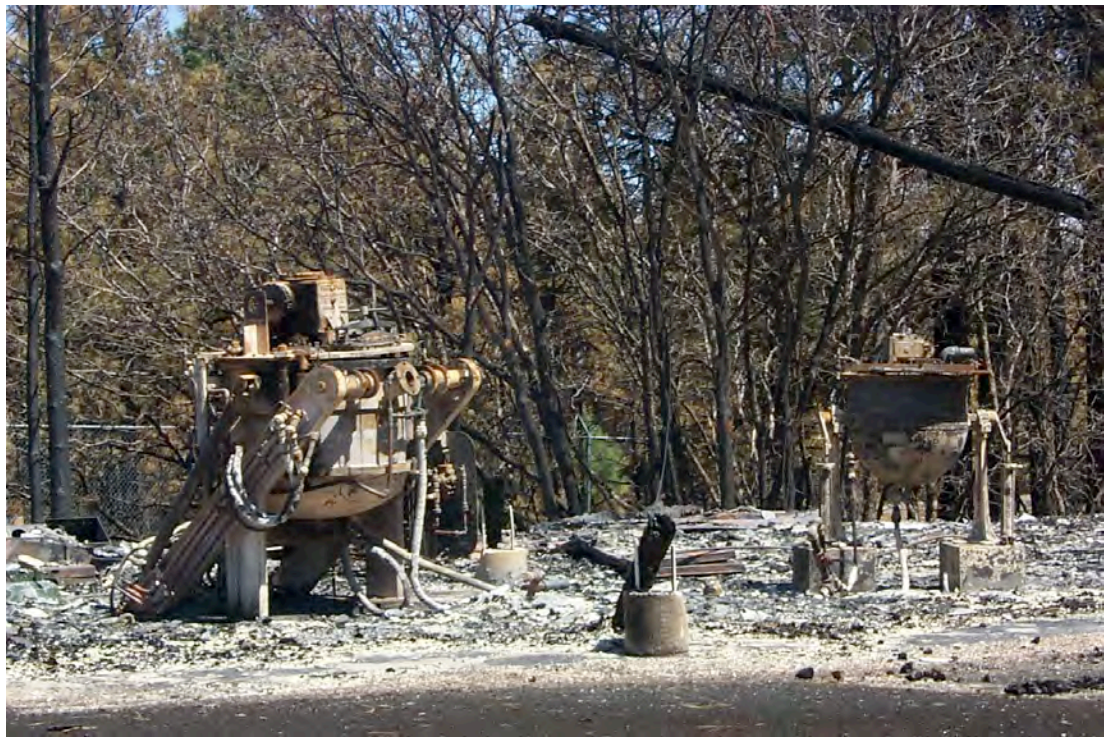
Figure 21.3. Candy kettles used to mix high explosives are seen here after the Cerro Grande fire.
