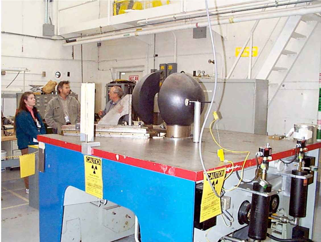
Figure 14.4. "Flattop" criticality assembly apparatus at TA-18.
