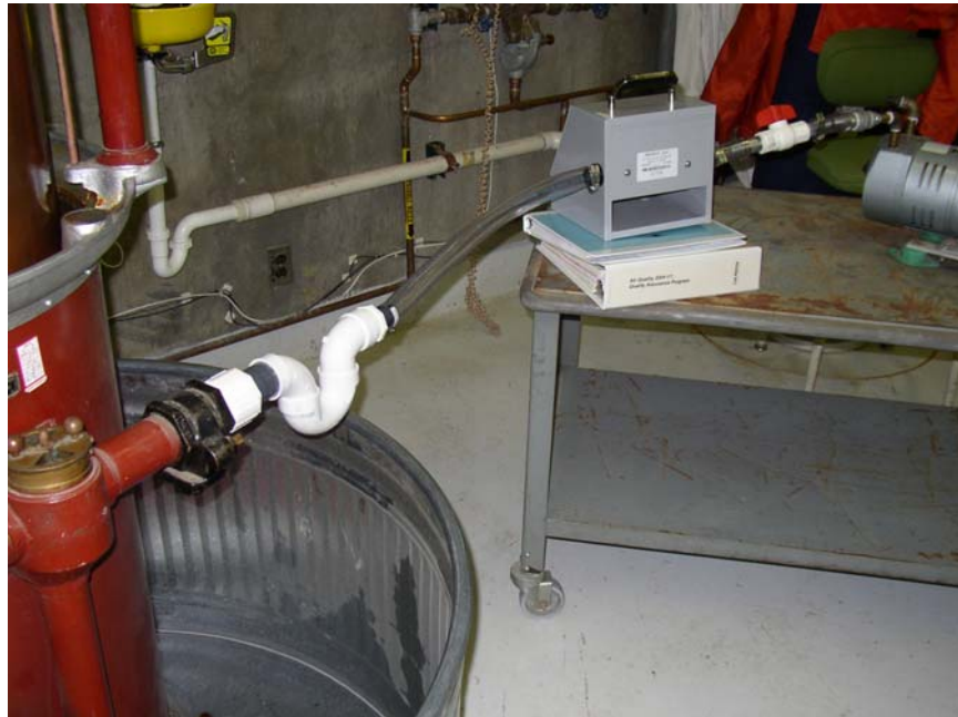
Connection of the hoses from the bell prover to the pump
