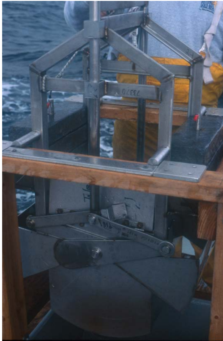
Customized box-core sampler used for the USGS sampling campaign on San Pedro Shelf in December 2004. Photo by C. Higgins
