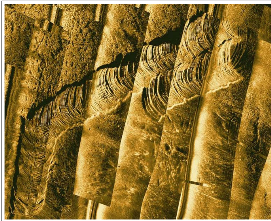
FIGURE 4. Mosaic of dredging scars compiled from high-resolution 600 kHz sonar images (Image courtesy of Marine Sonic Technology and Ocean Star Systems).
