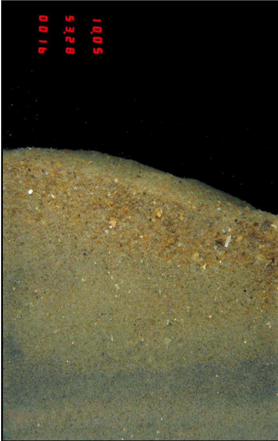
Figure 6-16. Sediment profile image from Station 20, Area 1, May 1998, Survey 1; note that grain size is similar to that of other images, but prism penetration is greater, which is a function of lowered sediment shear strength (image width represents 15 cm).
