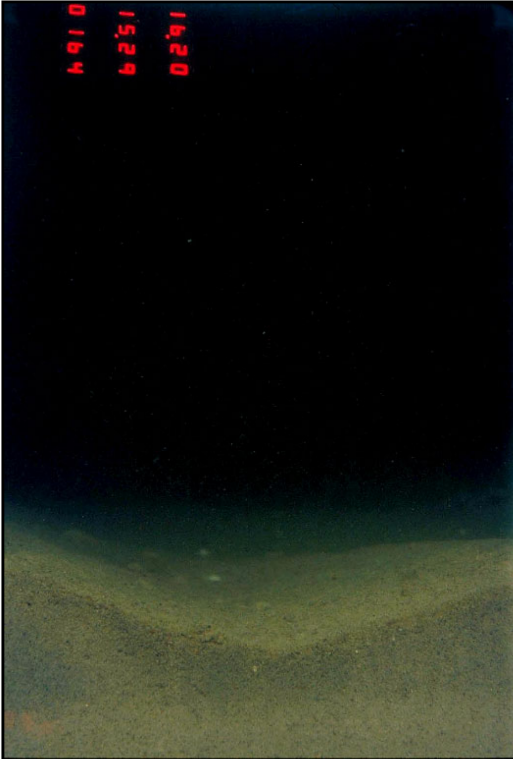
Figure 6-23. Sediment profile image from Station 1, Area 2, May 1998, Survey 1 showing the presence of bedforms and a grain size major mode of 4 to 3 phi (image width represents 15 cm).
