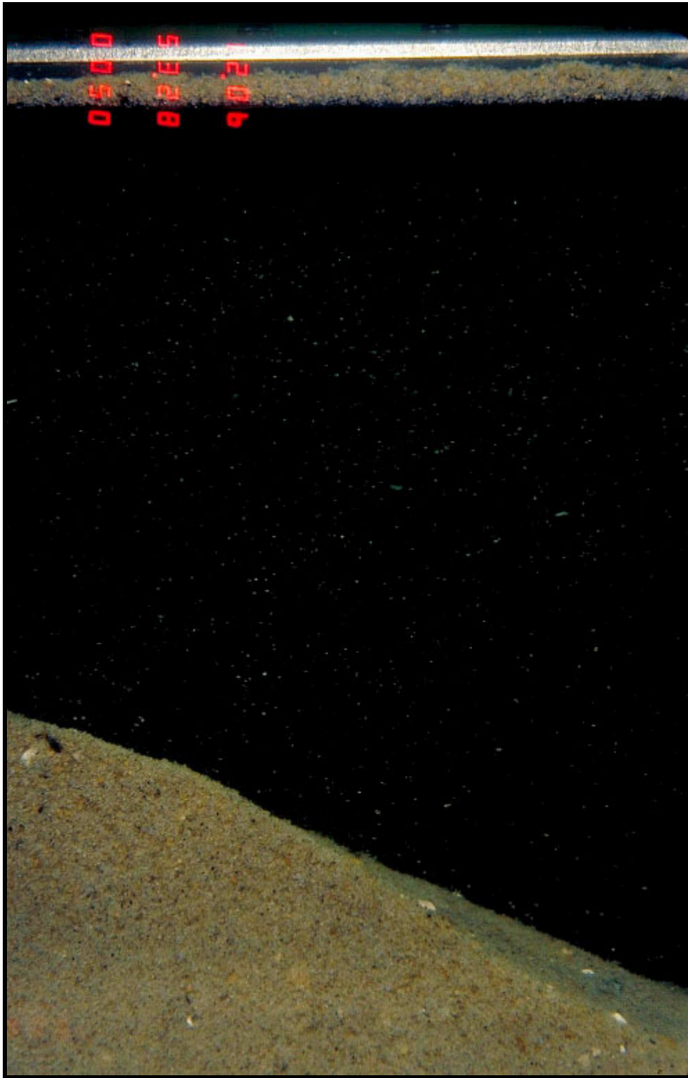
Figure 6-15. Sediment profile image from Station 13, Area 1, May 1998, Survey 1; boundary roughness values from all images in Area 1 were primarily due to surface relief from the physical forces that created the sand ripples present throughout the area (image width represents 15 cm).
