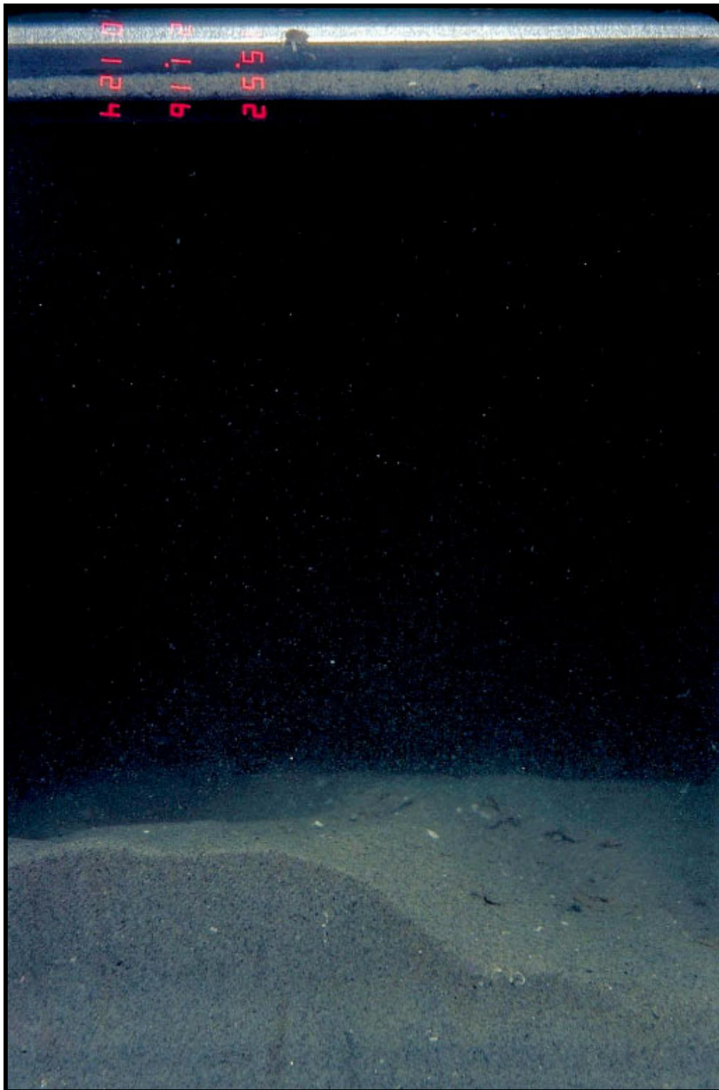
Figure 6-21. Sediment profile image from Station 2, Area 1, September 1998, Survey 2 showing surface roughness elements caused by infaunal burrowing activity; the crater-like rim of a large burrow opening can be seen in the left background of the image (image width represents 15 cm).
