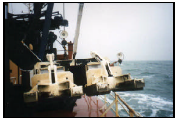
Plate 4.3.1b 'California' Type draghead fitted to the ARCO Dee with two underwater cameras and three water sample positions
