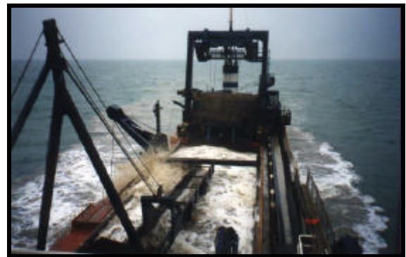
Plate 4.3.2 View astern of the ARCO Dee showing the smaller plume formed by this size of vessel.
