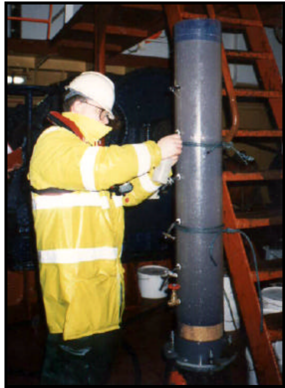
Plate 5.3 Measuring settling velocity aboard the ARCO Severn
