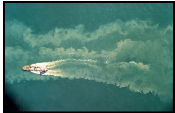
Plate 4.2.2.9b Multiple sediment plumes formed by successive passes of the TSHD Sand Harrier. The plume is less than 70m wide, 100m astern of the dredger. Sampling data from this study would indicate that suspended solids concentrations at the far right hand side of the picture would be approaching background conditions
