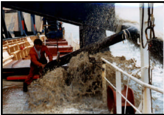
Plate 4.1.4 The practicalities of sampling the screened-off material from the reject chute
