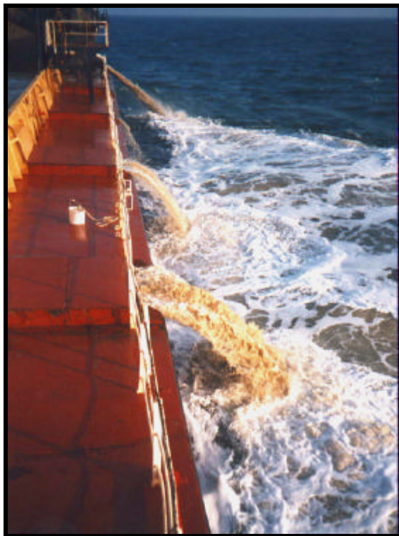
Plate 2.2.1c Overflow from the ARCO Severn
