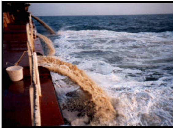
Plate 4.1.3 Sampling from the overspill
