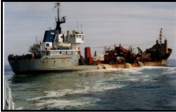
Plate 4.2.2.9a TSHD City of Rochester nearly completing loading a screened cargo at anchor, English Channel, August 1995. Monitoring of the plume from this vessel indicated that suspended solids concentrations were largely returned to background levels within 300-500m downstream. Gross plume was tracked for a further 3000m.
