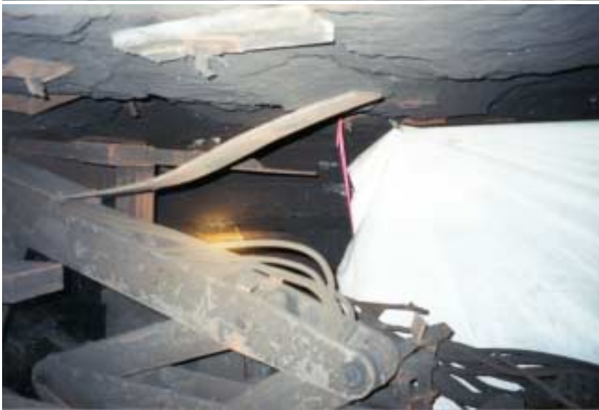
Figure 24: Standing on the left side of the roof bolter in the face of #4 entry. A thick metal cover is bent up and in toward the direction of the face.
