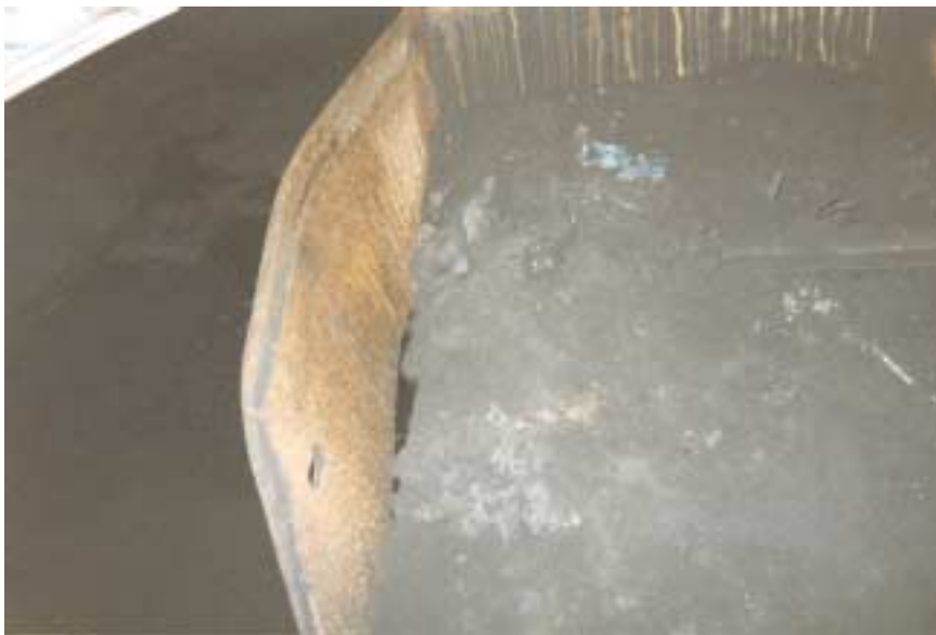
Figure 3: Damage to the outby side plate of scoop bucket.
