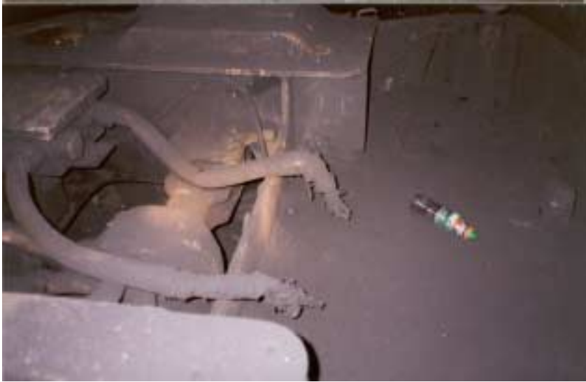
Figure 8: Battery end of scoop facing #1 entry. No battery and battery leads pulled loose from battery. Scoop located at spad #13352 toward #1 entry.
