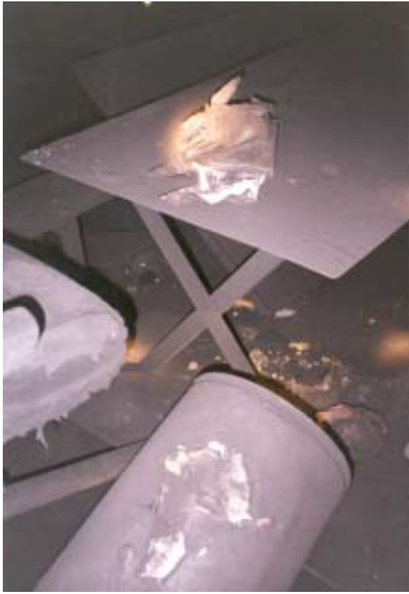
Figure 28: Located near the outby left corner at spad #13348. Picture of the effects of heat on trashcan, edge of seat and a book on the table.
