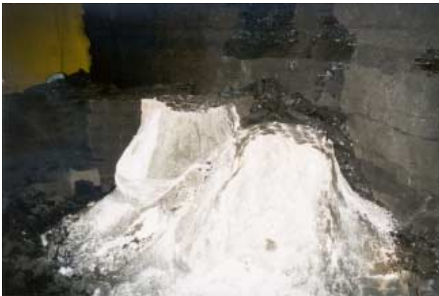
Figure 38: Located in the #2 entry and in the area of the rock fall along the inby ribline in the crosscut between spad #13333. Picture of two big rock dust bags melted or burnt away exposing dust.
