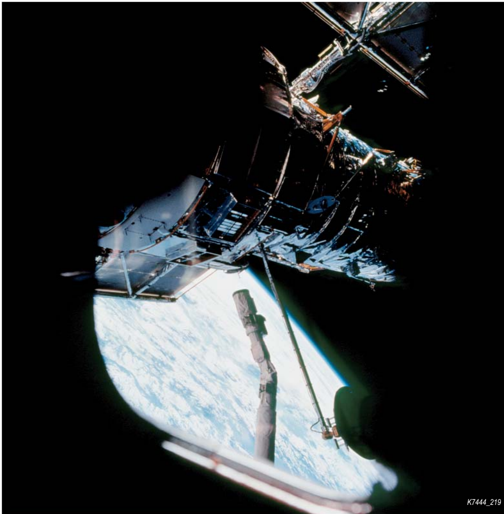
Fig. 2-19 Viewed through an overhead window on the aft flight deck of Space Shuttle Columbia, Hubble (partially obscured) begins its separation from the orbiter as it is released from the robotic arm. The STS-109 crew redeployed the giant telescope on March 9, 2002, at the close of Servicing Mission 3B.
