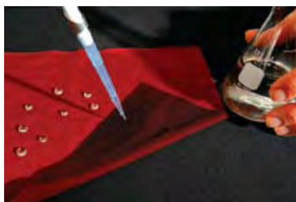
The new fabric treatment can produce water resistance on one side (see water droplets) and wicking on the flip side.
