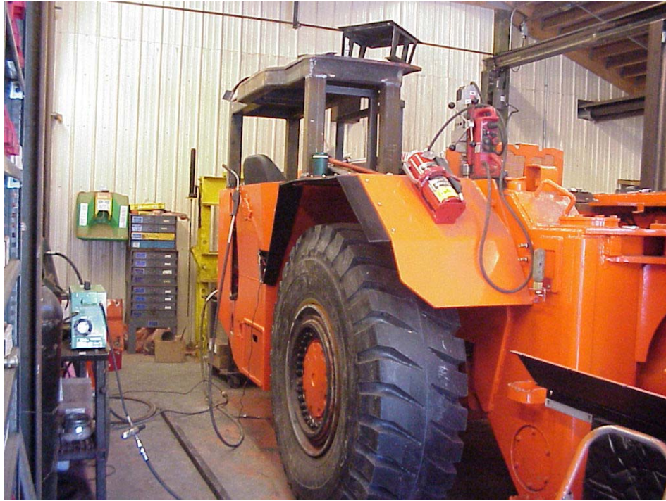
Figure 2. Cab Retrofit at SSX Mine.
