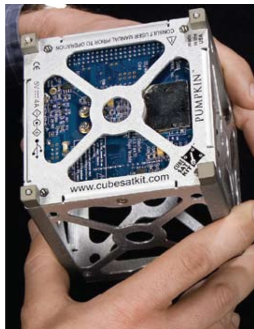
A cube sat is being prepared for launch.
