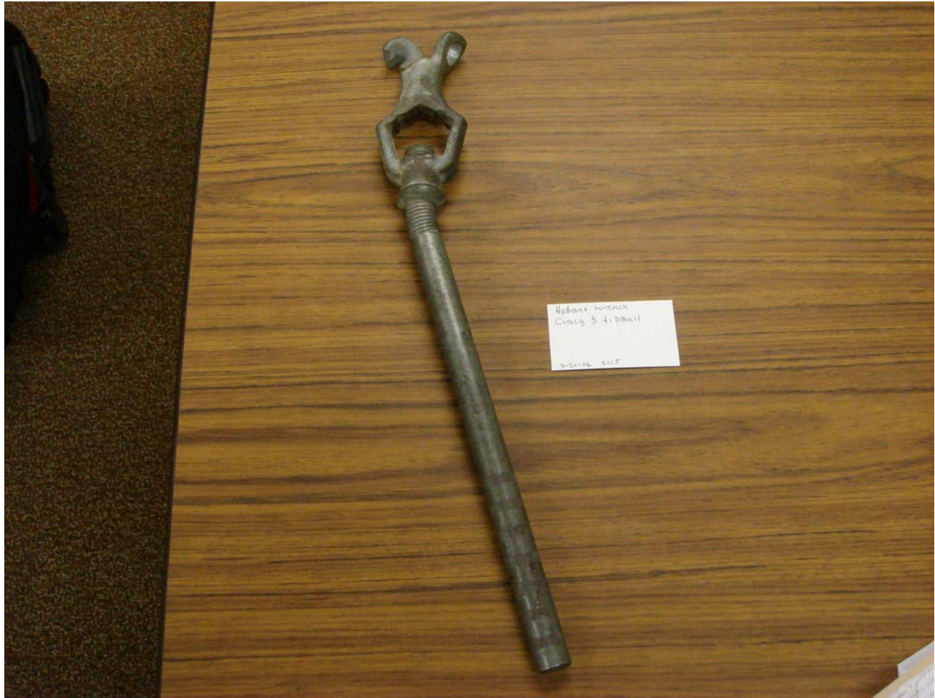
Photo 4. Bent hydrant wrench. (NIOSH photo)
