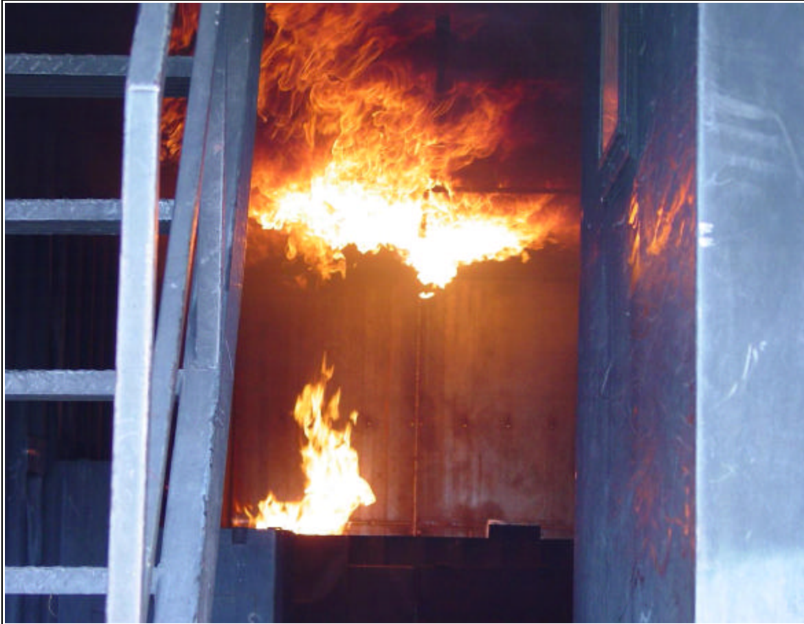
Photo 4. View thru rear doors showing cabinet prop at lower left and flashover bar at ceiling ignited. Dividing partition walls have been swung out of the way.
