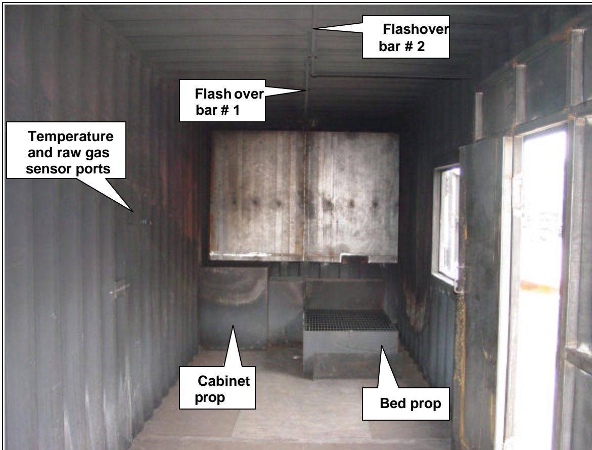
Photo 1. Inside view of front of burn chamber
